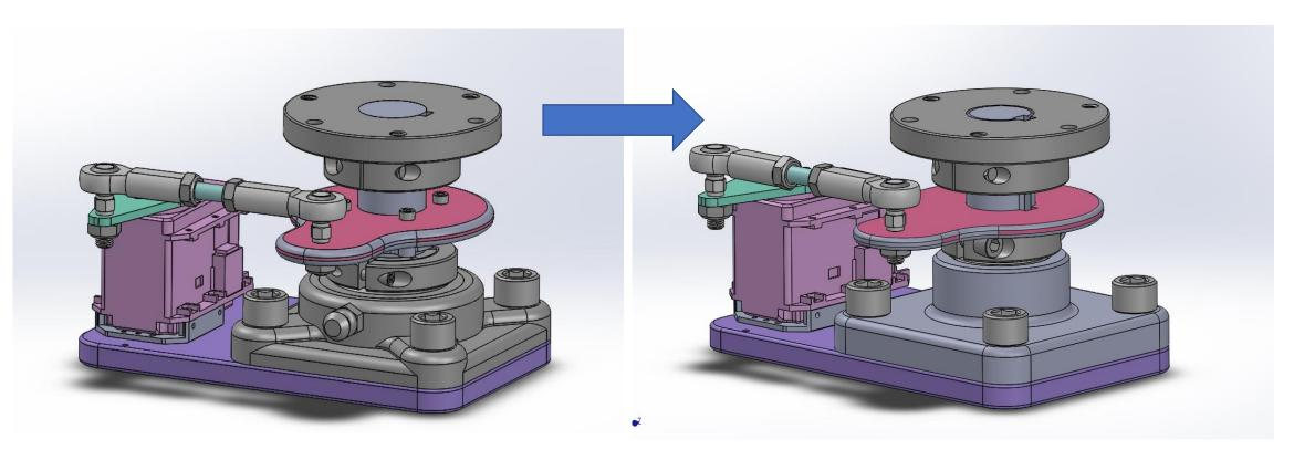
• Fixes both issues of bearing popping out of housing, and parts rotating about shaft due to resistance of foam. \*\*McMaster Carr will refund us for bearing if we send it back (will save us \$108)
