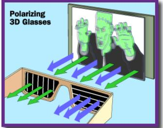
Our team is using polarized technology in conjuction with polarized projectors and a special silver projection screen to learn more about how this process works. Using linear polarized 3D glasses we network two projectors with similar filters and project both images onto a screen. Then using the keystone adjustments on the projectors we can overlay the two images on top of each other.
